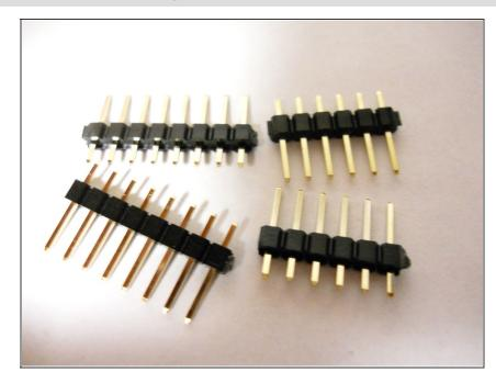
• From the 36-pin header, clip two 8pin and two 6-pin headers.
